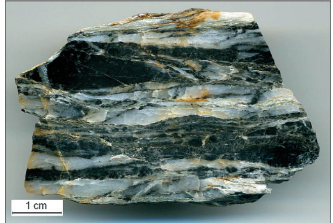
Text-Fig. 6. Banded tourmalinite, alternating quartz and tourmaline layers. Hand specimen, sample 72, trench 7.
