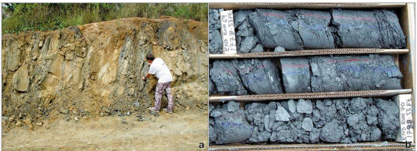
Text-Fig. 28. a) Steeply dipping graphitic schist on the Nyameani – Beposo road, near the village of Brodekwano (with P. CLAEYS, University of Brussels, for scale). b) Deformed or brecciated graphitic schist in the deep crater fill, as seen in deep borehole BH7, drilled in 2004, in the form of monomict autochthonous breccias (the image shows a portion of the core drilled at a depth between 542 and 545 m below lake level).
