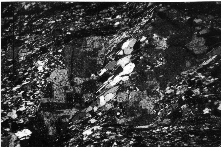
Text-Fig. 7. Rigid broken plagioclase crystall. Albite and quartz annealed the antithetic fracture. Zentralgneis sample of the Northern Sulzbach body near Hopffeldboden/Obersulzbachtal. Length of scale bar 1 mm, x-Nicols.
