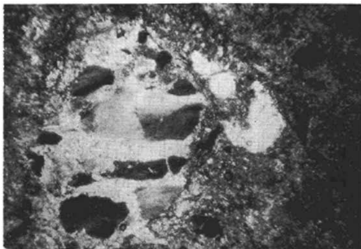
Photo 1. Effects crushing on quartz megacrysts in quartz porphyroid ( \times 15 ).
