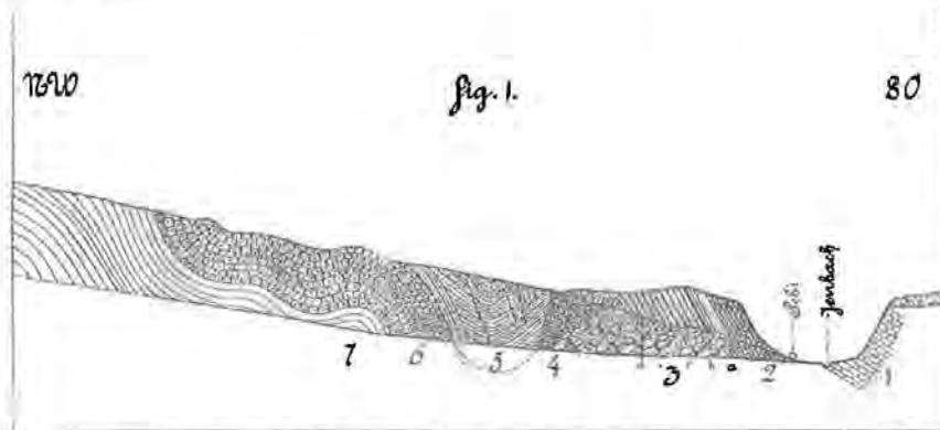
1 = Flysch; 2 = obere Kreide; 3 = oberer Lias (a dünngeschichteter Kalk, b rothe Zwischenlage, c grauer Kalk, d Crinoidenkalk); 4 = Berrias-Schichten; 5 = Hossfelder Schichten; 6 = graue Aptychenschiefer; 7 = bunte Aptychenschiefer.
