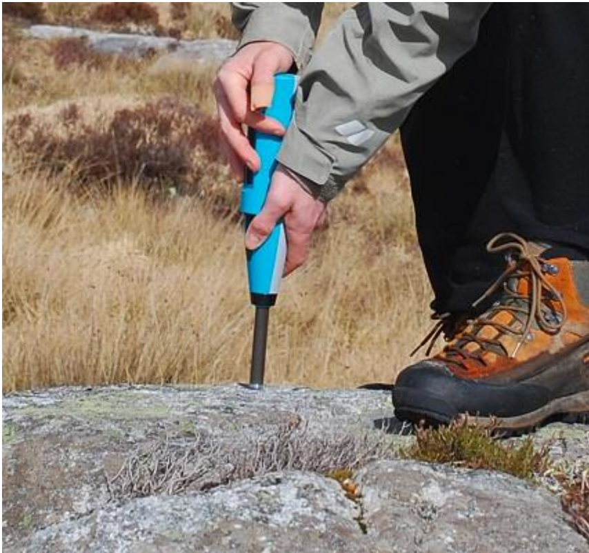
Figure 1: A Rocks Schmidt hammer being used to measure surface hardness (Rebound value) of glacially abraded granite bedrock in the field.
