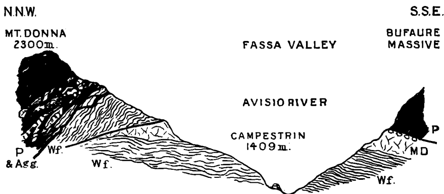
FIG. 15.—Section through Fassa Valley (between Fontanazza and Campestrin). Wf. = Werfen marls and marly limestones; MD. = Mendola Dolomite; P. = Augite Porphyrite; P. & Agg. = Porphyrite and Contact Breccia, the enclosed fragments are mostly Mendola Dolomite (Scale 1:25,000).
