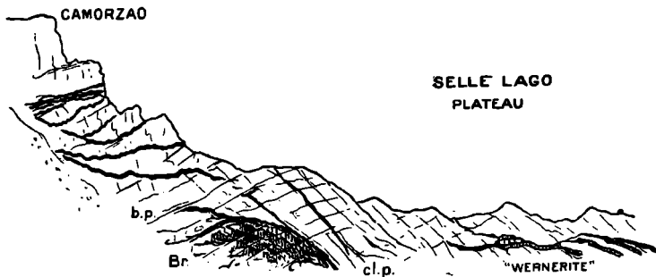
FIG. 27.—Camorzaio escarpment and plateau. Intercalated system of porphyrite dykes. Contact minerals well developed, the "Wernerite" locality being rich in ores. Br. is a contact breccia of dyke and limestone, the threads of the magma have ascended both cleavage and bedding-planes, and the appearance is that of a lenticular meshwork surmounted by an "arch" of stratified rock, the apparent domal shape is here the result of injection along planes intersecting almost rectangularly.
