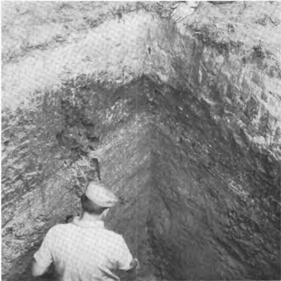
8. Impermeable quaternary loam, light grey on top, dark grey below, covers weathered solifluction in test pit S 5
