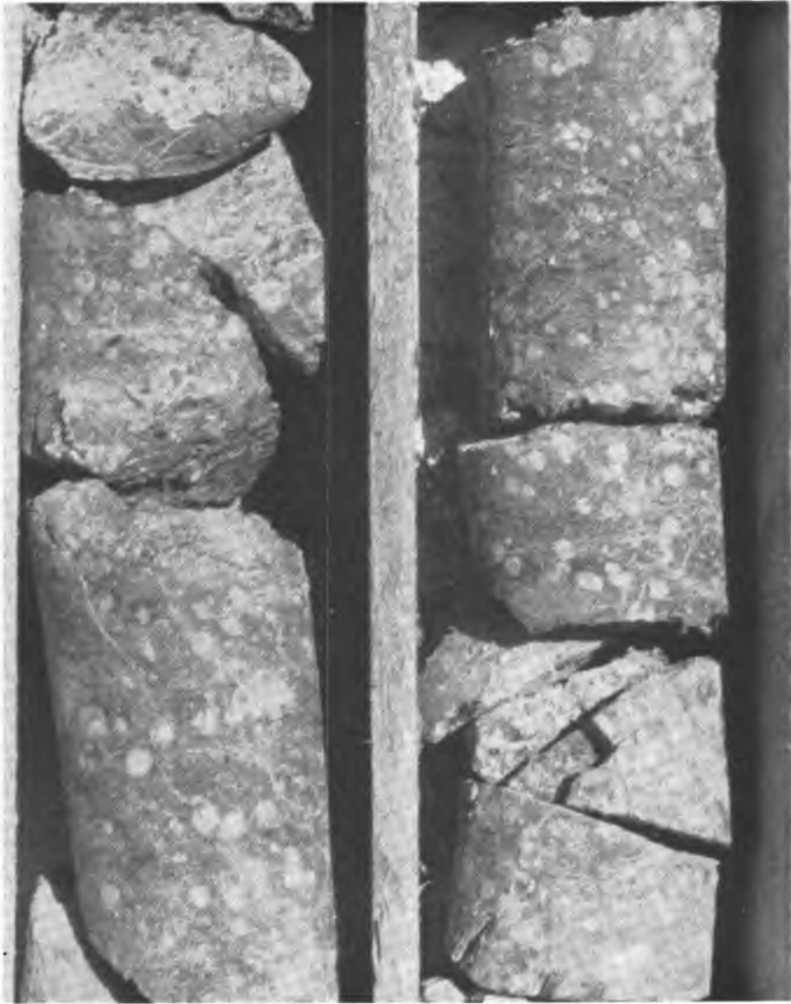
15. Cores of serpentine rock. drilling 1967/a, 17—19 m
