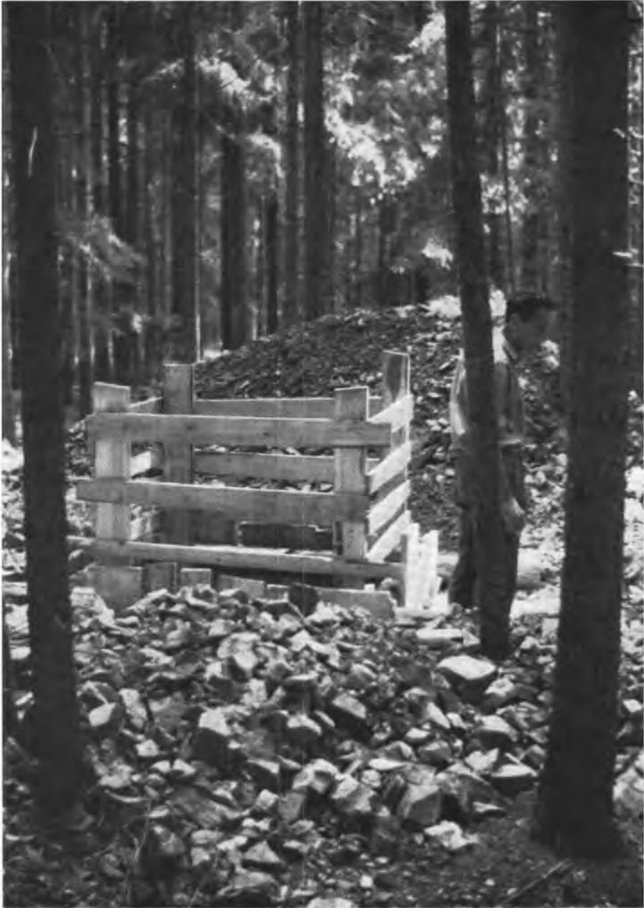
6. Test pit S 11 reached unweathered granulite
