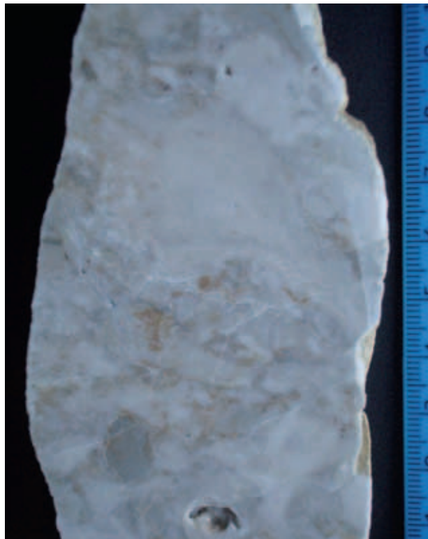
Fig. 11: Polished slab of clast-supported carbonate breccia constituted of light clasts ranging in size from a few mm to 3-4 cm. Scale is in cm
