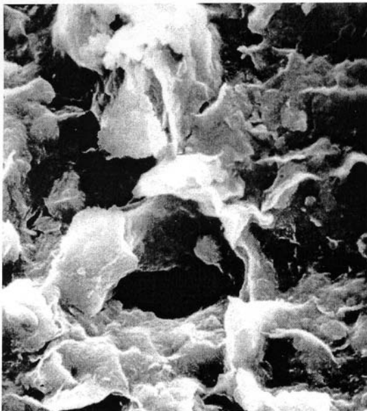
Fig. 7: REM image of kaolinitic clay, scale 5000x. High non communicating microporosity, electrically neutral two layer mineral without swelling potential. Preferable mineral phase for surface sealing.
