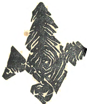
Fig. 26.—Skeleton rhombohedron of titaniferous iron, Crossall Hill, Dalmeny (magnified 20 diameters).
