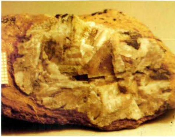
Fig. 6: A several cm large elongated nodule composed of coarse, lath-like barite crystals embedded in fine-grained red karst sediments (Streitegg Alm).
