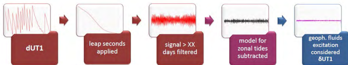
Figure 6.1: Signal preprocessing scheme for the calculation of zonal tidal variations from dUT1.
