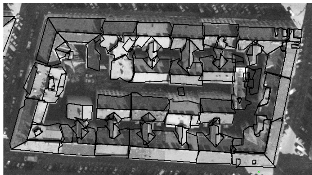
Figure 6.6: Roof polygons of the building in figures 6.2, 6.3, and 6.4 back projected to an aerial image. Ground sampling distance: 17 cm.
