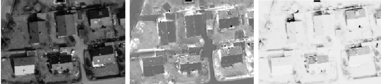
Figure 5.6: Intensity of the CIR image (left), NDVI (centre) and \sigma_{NDVI} (right) for a part of the Memmingen data set. In the \sigma_{NDVI} image, white areas correspond to low \sigma_{NDVI} .
