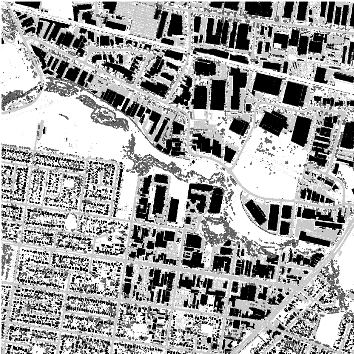
Figure 4.6: The results of the initial Dempster-Shafer classification. White: grass-land ( G ), light grey: bare soil ( S ), dark grey: trees ( T ), black: buildings ( B ).
