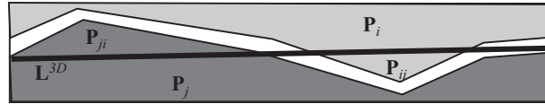
Figure 7.2: Two planes \mathbf{P}_i , \mathbf{P}_j . \mathbf{P}_{ij} is cut off \mathbf{P}_i by the intersection line \mathbf{L}^{3D} , and \mathbf{P}_{ji} is the part of \mathbf{P}_j cut off by \mathbf{L}^{3D} .
