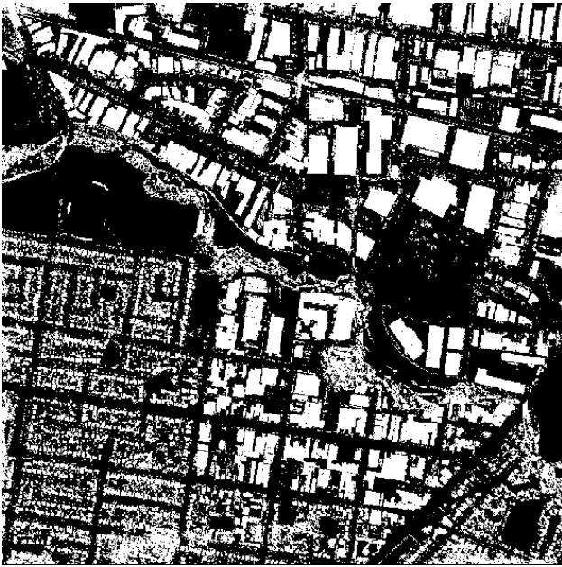
Figure 3.4: The initial building mask corresponding to the left DTM in figure 3.3. The residential buildings on a small hill at the southern border are merged.
