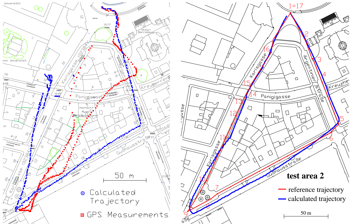
Fig. 5. Urban test area in the 4 th district of Vienna with DRM III Trajectory (left) and NAVIO multi-sensor system trajectory (right)
