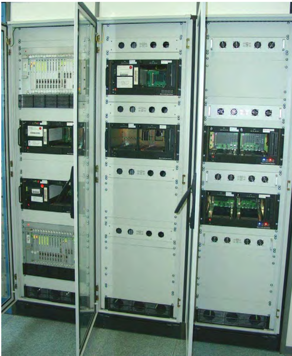
Figure 1. Correlator at Bonn. Racks with (from left to right): two SUs + two Mark 5A, two Mark 5A + the space for four CIBs and two Mark 5B + the space for four CIBs.
