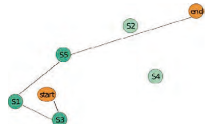
Fig. 2: Example of a path cost for the branch and bound algorithm: \text{path cost}(S5) = \text{distance}(\text{start}, S3) + \text{duration}(S3) + \text{distance}(S3, S1) + \text{duration}(S1) + \text{distance}(S1, S5) + \text{duration}(S5) + \text{distance}(S5, \text{end})
