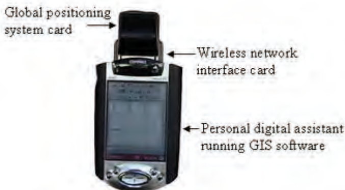
Fig. 3: A MoGeo device consists of a mobile computer (handheld or tablet), a global positioning system receiver, wireless access, GIS software, and communication software.
