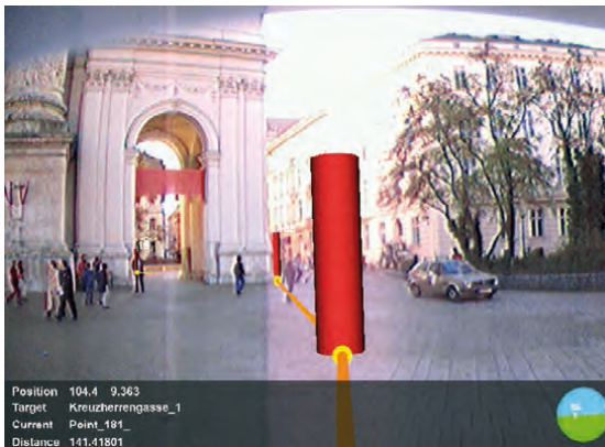
Fig. 5: An outdoor navigation guide for a pedestrian visualizes the selected route as a series of waypoints. Note the correct occlusion between the route and the archway .
