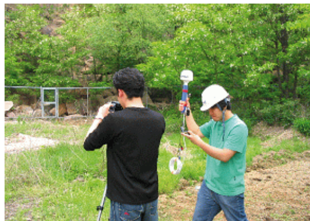
Fig.4: Digital image and spatial data acquisition using digital camera and DGPS
