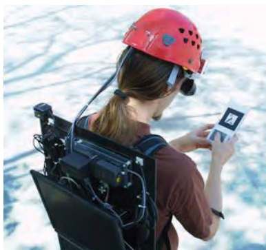
Fig. 1: The backpack system is based on a conventional notebook computer displaying stereoscopic graphics overlays in an optical see-through head mounted display.
