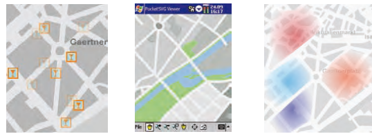
Figure 5: Relevance of POI encoded with opacity (left); colour-grey contrast (middle); hot-cold metaphor (right). (© base data: Städtisches Vermessungsamt München)
