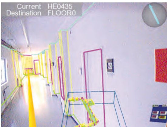
Fig. 7: Indoors, a combination of directional arrows, highlighting of exit, compass (upper right) and world-in-miniature (lower middle) is used to help a user navigate the environment.
