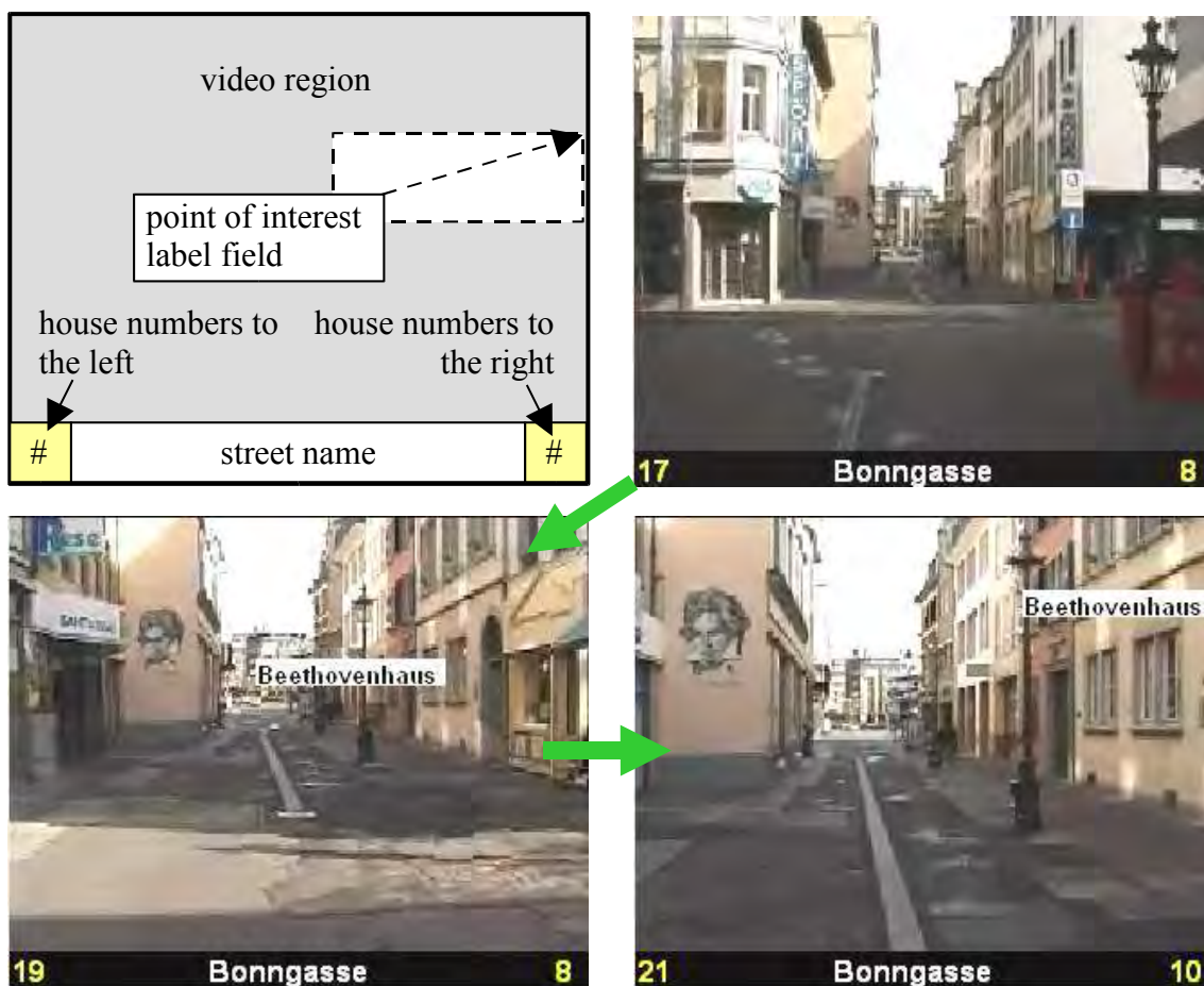
Fig. 4: Screen layout for and screenshots from the prototype for augmented video visualization using RealOnePlayer (Real 2002). The screenshots were taken at three points along the path to the "Beethovenhouse" in Bonn. Please note, that at a certain distance a label becomes visible which then moves within the video region.
