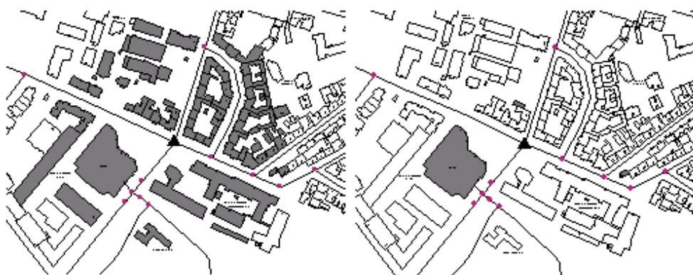
Fig.3: Scene of Hanover (road network with decision points, buildings) – left: “local environment” around chosen decision point (created by a buffer), right: potential landmarks after processing
