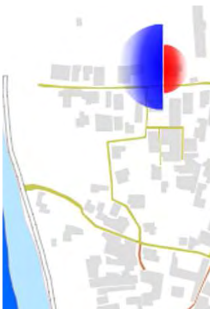
Fig. 3 (above): Example of a RIM dynamic risk symbol showing the modelled risks (blue for floods, red for earthquakes) at the current pointer location.
