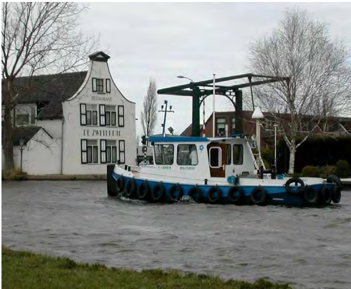
Fig.1: The small boat, with several GPS receivers and antennas on-board, all collecting measurements simultaneously, was cruising the Schie-canal forth and back for an almost 3-hours period. The boat is depicted here at the little village De Zweth.
