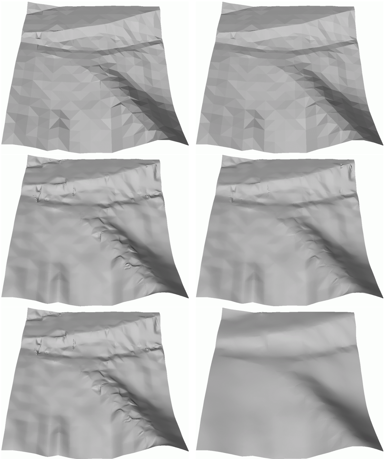
Figure 5.9: Subdivision with interpolating and approximating paraboloids. Upper left: original data, Upper right: original data after removal of random errors with kriging, Lower left: purely interpolating scheme on the original data, Lower right: purely approximating scheme on the original data, Middle left: scheme with interpolation for the original points and approximation for the newly inserted points on the original data, Middle right: interpolating/approximating scheme like on the left side but on the triangulation after removal of random noise.
