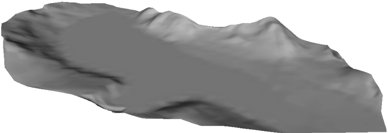
Figure 6.12: Gently sloping terrain surface reconstructed with an interpolating/approximating subdivision approach based on paraboloids as local surfaces.
