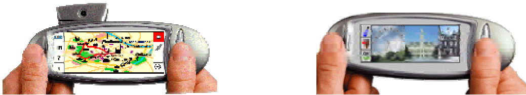
Fig. 6: Lol@ - Interface (by using a design-draft for a UMTS-device of Nokia; left figure: Reference Map Interface; right figure: Multimedia-Content-Interface)
