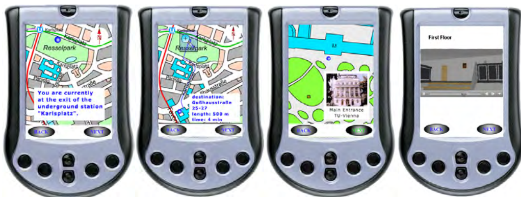
Fig. 7: Different animated multimedia route presentation forms, linked in a Pedestrian Navigation System for a mixed indoor/outdoor environment: Application draft for TU Vienna - LBS
