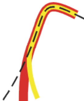
Fig. 4: Complex Line-Styles composed of three lines sharing the same geometry, but with different line-styles. source: (WINTER, NEUMANN, 2001)
