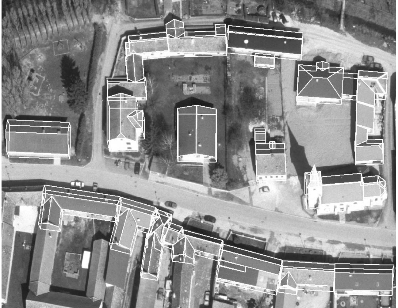
Figure 7.8: A part of one of the digital images used for reconstruction with all the reconstructed buildings super-imposed to it in white colour.
