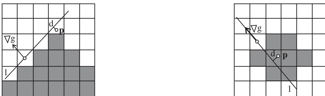
Figure 5.4: Two point models. Left: a corner point. Right: a circular symmetric point. The point \mathbf{p} is computed from an intersection of all lines l by least squares adjustment.
