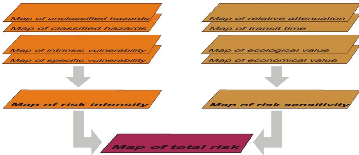
Fig. 35: System of risk maps showing the hierarchical structure of the different type of maps.
