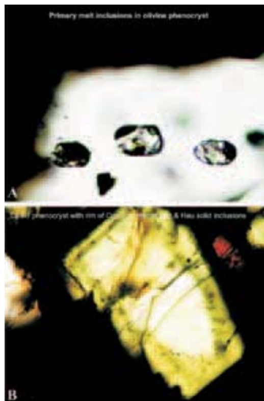
Figure 30 - A) Primary composite inclusions in olivine phenocryst: melt + diopside, S and CO 2 ; B) Zoned clinopyroxene phenocryst: the internal part has a primary composition and is surrounded by a late stage crystallisation clinopyroxene. The rim clinopyroxene contains inclusions of apatite and haüyne.
