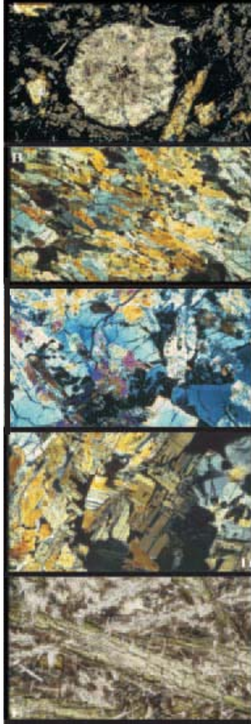
Figure 6. - A) Calcite-zeolite filled ocelli in the eumite body; B) melilite euhedra poikilitically enclosing wollastonite; C) anomalous blue-grey interference colours and yellow rims on melilite; D) anorthite globular structure; E) quench diopside with aegirine rims in a groundmass of glass, leucite, anorthite and melilite.
