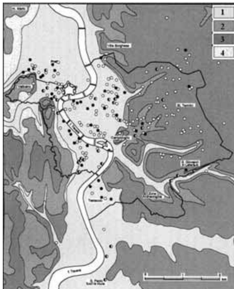
Figure 2.3 - Effects of the 1915 Fucino earthquake in Rome, overlapped on a simplified geological scheme (modified, after Molin et alii, 1995). Buildings sited above the Holocene alluvial deposits suffered most of the damage. 1: Holocene alluvial and marsh deposits, 2: Pleistocene alluvial and marsh deposits, 3: Volcanics, 4: Pliocene marine deposits (shale and sand).
