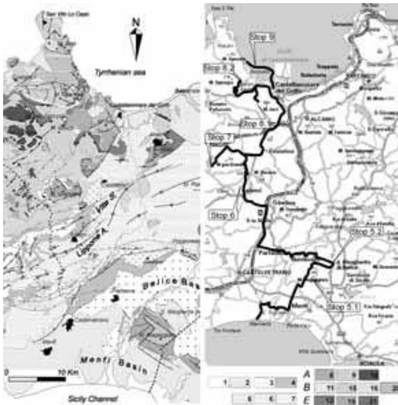
Figure 25 - Geological (left) and road map right with the 2 nd day itinerary. 1) Recent; 2) Clastic carbonates, Pleistocene-Pliocene; 3) Marls and calcarenites, Pliocene; 4) Trubi, e. Pliocene; 5) Evaporites, Messinian; 6) Reef carbonates and Terravecchia Fm.; l. Messinian-U. Tortonian. A) Pre-Panormide Units: 8) Shelf Lms., l. Miocene; 9) Shales and sandstones, l. Miocene - Oligocene; 10) Marly calcilutites, Eocene - Cretaceous. B) Panormide Units: 11) Glauconitic calcarenites, e. Miocene; 15) Shelf to slope Lms., Cretaceous - Oligocene; 16) Pelagic Lms., Jurassic - e. Cretaceous; 20) Platform Lms., Triassic - Lias. E) Trapanese Units: 12) Sandy marls, l. Miocene; 19) Pelagic platform deposits, Oligocene - Jurassic; 21) Platform carbonates and dolomites, Lias - Trias.
