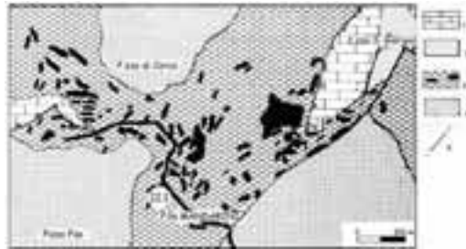
Figure 46 - Simplified geological map at Portella di Mandarini. Mesozoic dolomites (1), Cretaceous-Eocene marly lms. (2), silty clays and arenites with carbonate megabreccias (3), followed by Li. Miocene quartzarenites and silty clays (Numidian Flysch) (4) pertaining to the Quacella tectonic unit.
