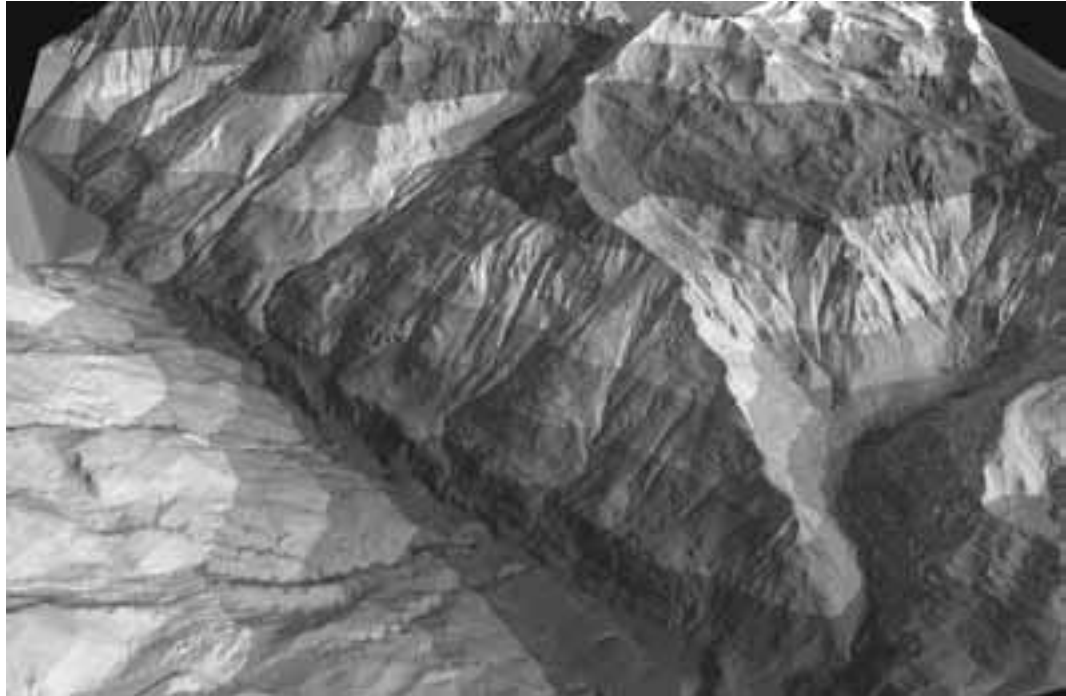
Figure 43 - DEM of the middle Susa Valley with Clot Brun large slope instability (central part of the image, left side of the valley).
