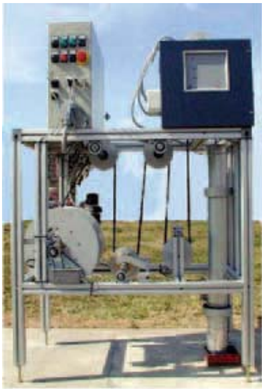
Figure 15 - Automatic Inclinometer System instrument.
