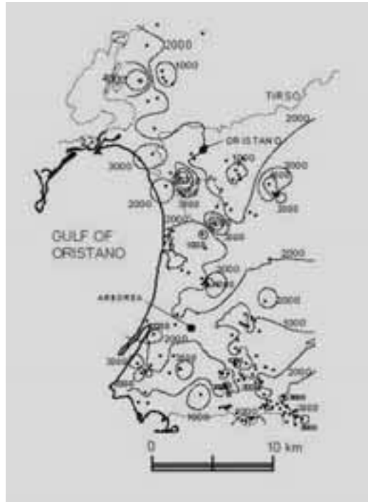
Figure 31 - Isosalinity curves ( \mu\text{S}/\text{cm} ) for the surface aquifer (after Salis & Soddu, 2003).
