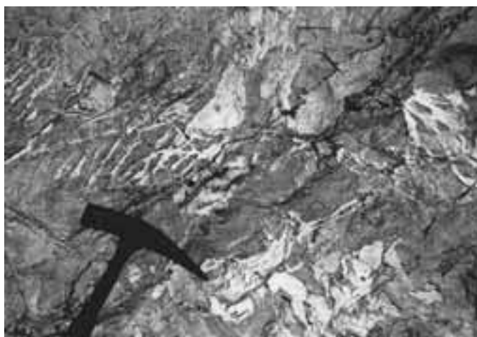
Figure 5 - Paleokarst collapse breccia and cockade ores with calcite, barite and Ag-rich galena. San Giovanni mine, Scavi Peloggio
