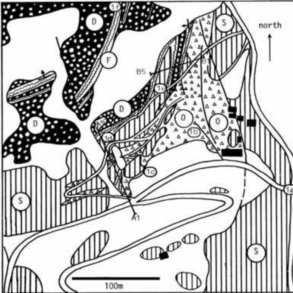
Figure 11 - Geologic map of the area around the contact between serpentinite breccia and massive basalt, Cava Galli-Mt. Rossola (SE slope), along the trail. Symbols: S: massive serpentinites; O: ophicalcite breccias; F: ophiolite sandstones and red siliceous shales and siltstones; D: massive basalt (after Abbate et al., 1980).
