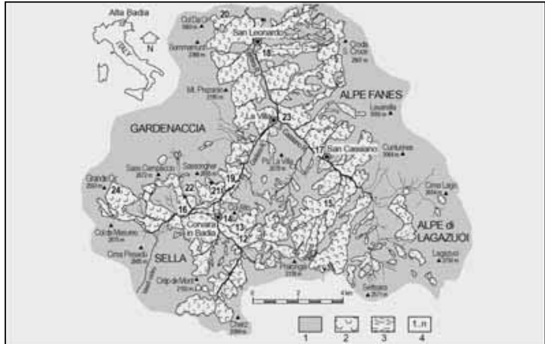
Figure 18 - Geomorphological sketch of Alta Badia area (heights are given in metres). Legend: 1) bedrock; 2) landslide; 3) lacustrine deposits; 4) landslide numbering according to Table 2 (after Soldati et al. , 2004).
