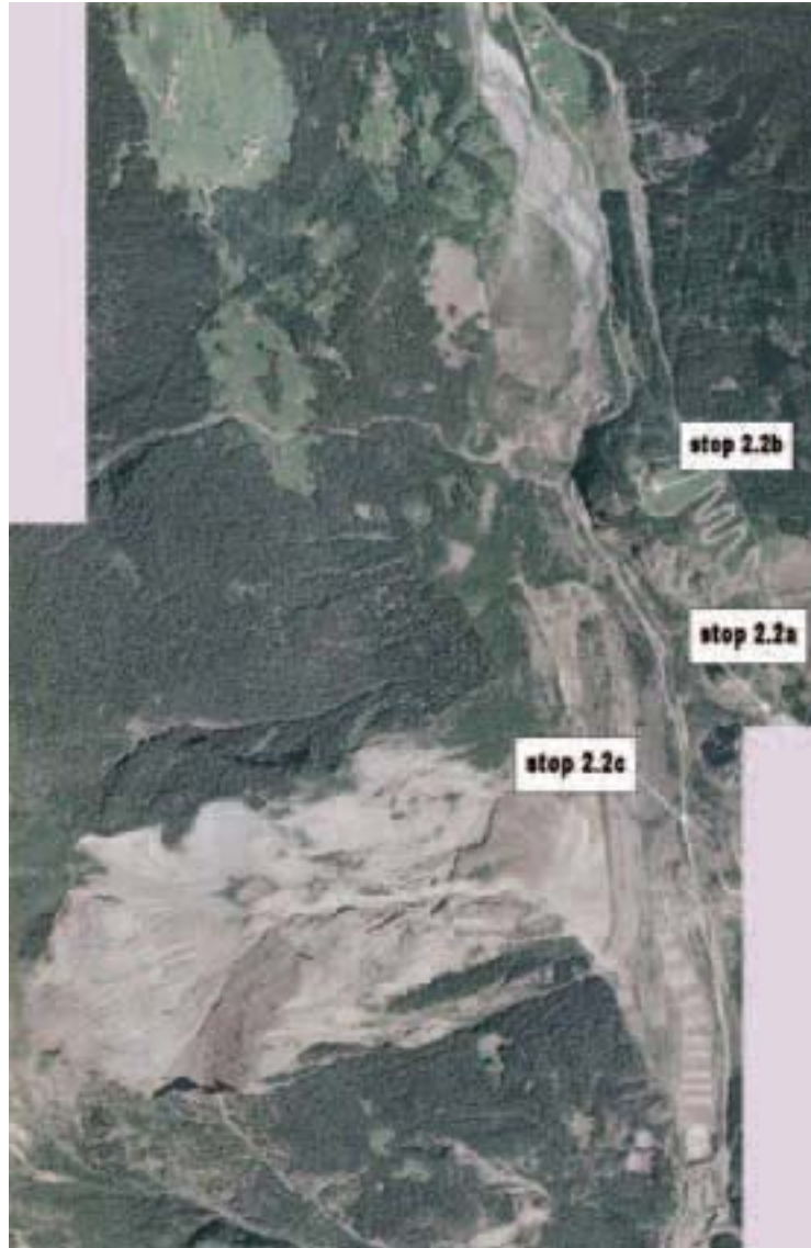
Figure 30 - Orthorectified photography (1999) of the Valpola landslide area, showing the stops. In the lower part the whole rock avalanche area is visible, as well as the repairing works. The upper part of the picture shows the area that was flooded by the ValPola lake, after the main event.
