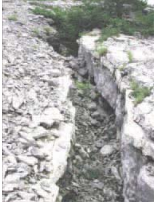
Figure 65 - a) An example of tension crack affecting the outcropping limestone formation. The instability phenomena are mainly related to the low shear strength of the clayey-marly interbeds. b) Buckling structure in the slide surface of Lavini di Marco landslide, involving a package of plane layers (about five meters thick).
