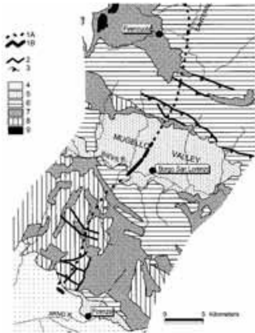
Figure 1 - litotechnical sketch along the Tuscan stretch of the new railway line 1A=tunnels; 1B=open air stretches; 2=faults or master joints; 3=thrusts; 4=alluvial deposits; 5=fluvio-lacustrine deposits; 6=Flysch-facies formations (alternating sandstones and marls); 7=mainly clayey formations; 8=marly limestones; 9=ophiolites.
