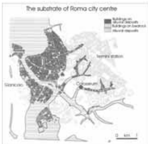
Figure 12 - Damage to buildings in Roma is essentially related to the type of substrate and the seismic impedance of alluvial sediments
