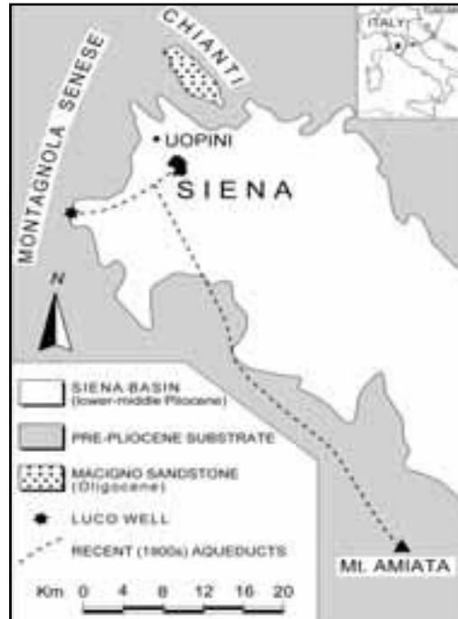
Figure 1 - Schematic geological map of the Siena Basin. A modern aqueduct was built during the early part of the 1900s getting water from Mt. Amiata (about 60 km from Siena). During the 1960s, waters from the Luco Well were added to augment the aging Mt. Amiata aqueduct
