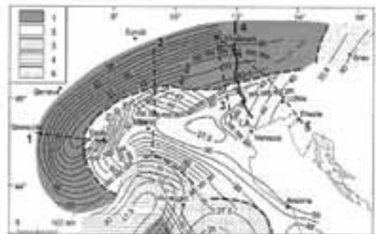
Figure 4 - Moho depth contours in the whole Alpine and North Italian region (from Cassinis et al., in press). Five crustal types are interpreted: 1=European; 2=Adriatic; 3=Transitional peri-Tyrrhenian; 4=Suboceanic; 5=Western corner of the Pannonian basin. Traces 1 to 5 of the five profiles of Figure 5 are located.
