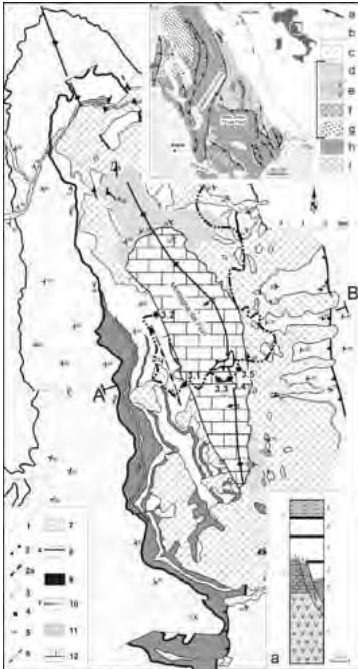
Figure 3.1 - Structural sketch map of the Montagna dei Fiori. The inset shows the tectonic sketch of the outer zones of the Central Apennines. The key to symbols is in Figure 1.1.: 1) Normal fault; 2) Thrust; 2a) Laga Detachment; 3) Backthrust; 4) Anticline axial trace; 5) bedding; 6) Itinerary and location of the stops (3.1 – 3.5); 7) Quaternary continental deposits; 8) Messinian Laga Fm.; X) Gypsum-arenitic layer; 9) Tortonian-Messinian Marne a Pteropodi Fm.; 10) Burdigalian-Tortonian Marne con cerroghna Fm.; Y) Calcareoclastic deposits; 11) Eocene-Oligocene Scaglia Cinerea Fm.; 12) Lower Lias-Eocene neritic-pelagic succession. A-B Trace of cross-section in Figure 3.2. a) Stratigraphic section of the Umbria-Marche succession. 1) Anidriti di Burano (Upper Trias); 2) Calcari e marne a Raethavicula e Calcare Massiccio (Upper Trias-Lower Lias); 3) Corniola, Rosso Ammonitico and/or Calcari e marne del Sentino (Upper Sinemurian-Aalenian); 4) Formazione del Bugarone (Pleisbachian-Lower Tortonian; in the condensed succession); 5) Calcari e marne a Posidonia, Calcari diasprini umbro-marchigiani, Maiolica, Marne a Fucoidi (Bajocian-Lower Cenomanian); 6) Scaglia bianca, rossa e cinerea (Middle Cenomanian-Oligocene); 7) Bisciario, Schelier, Marne con cerroghna, Marne a pterapodi (Aquitanian-Messinian p.p.); 8) Turbiditic siliciclastic deposits (Burdigalian p.p.-Messinian). The heavy lines represent: Rosso Ammonitico, Marne a Fucoidi and Scaglia cinerea-Marne con cerroghna Fms, from older to younger respectively.
