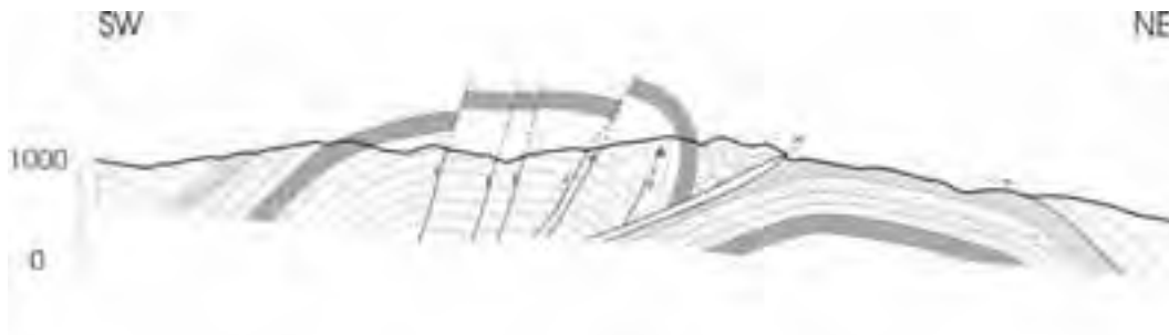
Figure 3.12 - Geological section across the Sibillini Mts Thrust. A- Pelagic condensed succession. Symbols as in Figure 3.11.
