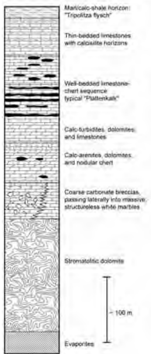
Figure 11 - Stratigraphic column of the Plattenkalk Group in central Crete, simplified from Hall and Audley-Charles (1983).
