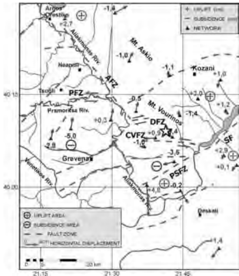
Figure 49 - Horizontal and vertical displacements of the distinguished blocks, based on GPS measurements for the period May 1995 - September 2000 (after Fountoulis et al., 2002).
