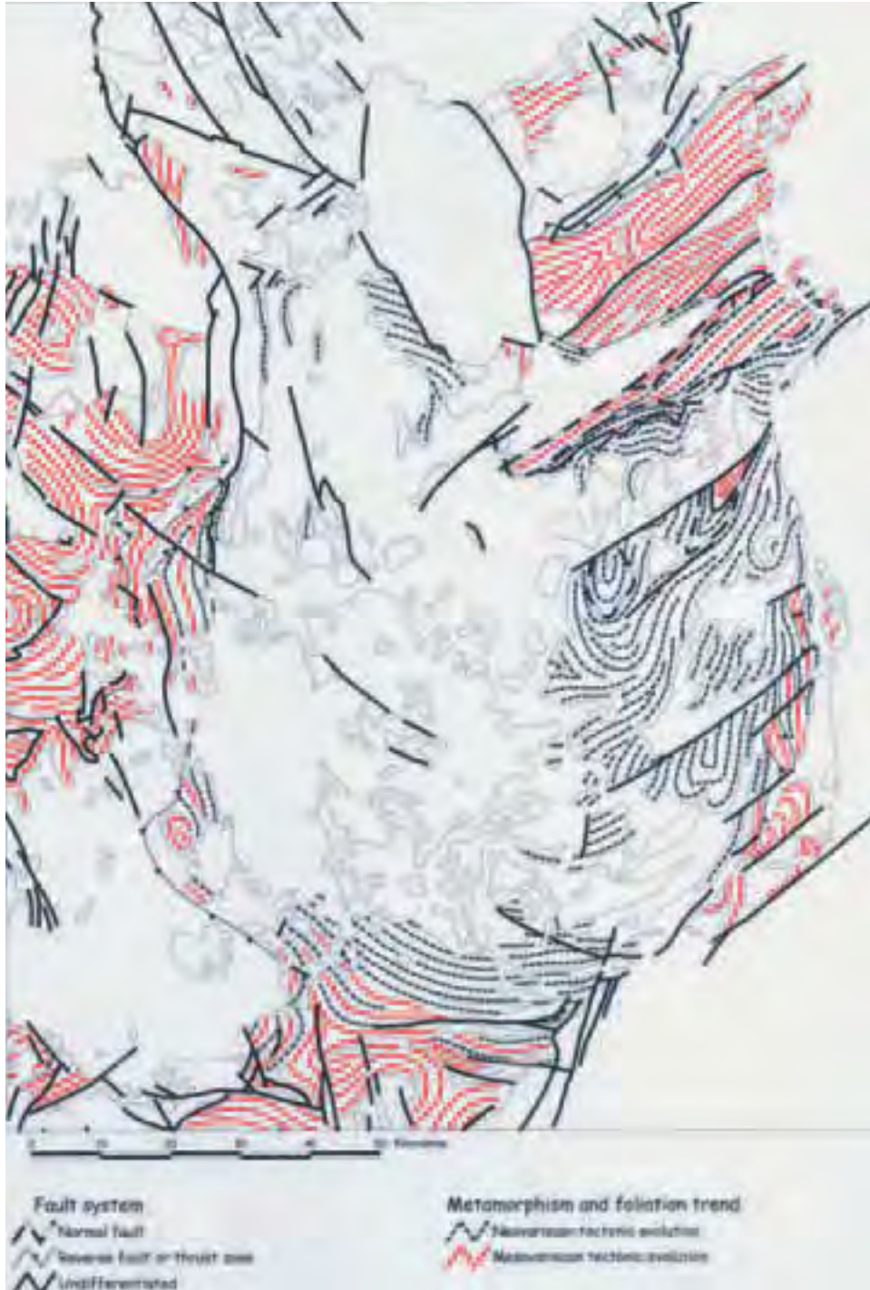
Figure 30 - Extension of Meso and Neovariscan metamorphism and foliation trends within the host rocks of the Velay migmatite-granite dome
