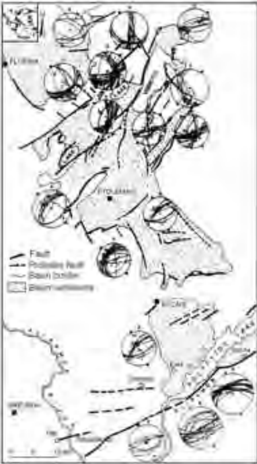
Figure 44 - Map of the Ptolemais - Servia - Florina Neogene-Quaternary basin showing the main faults. Equal-area projection of measured striated faults (after Mountrakis et al., 1998).
