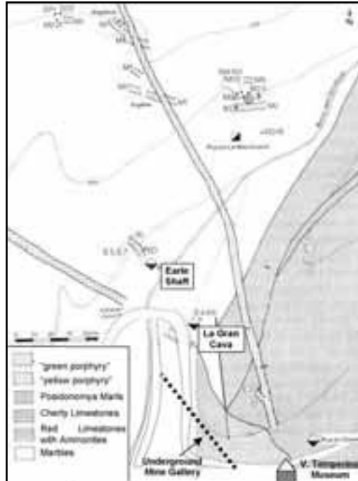
Figure 18 - Schematic geologic map of the Valle del Temperino deposit area (modified after Corsini and Tanelli, 1974)
