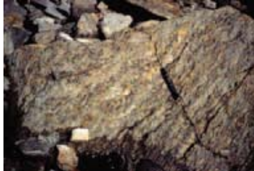
Figure 41 - Metapelitic schist from upper Zone 3. The light brown to orange nodules are polycrystalline aggregates of staurolite. See Figure 42 for a microscopic view of an aggregate from this rock.
