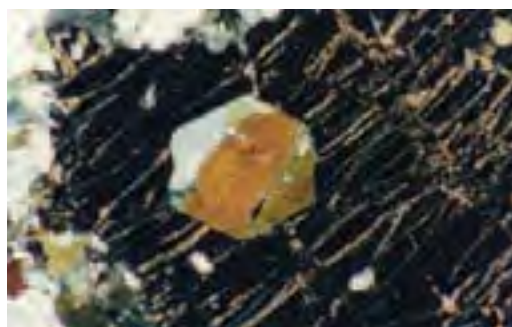
Figure 30 - Inclusion in garnet. The shape of the inclusion, a negative garnet crystal, and the composition of the mineral phases suggest that included minerals crystallized from a portion of trapped magmatic liquid.
