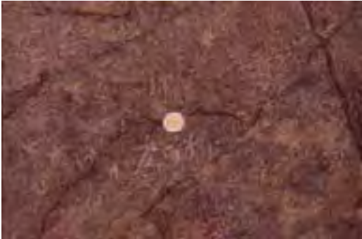
Figure 40 - Hand specimen of a graphitic schist from lower Zone 3, with abundant coarse-grained andalusite porphyroblasts.
