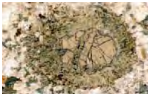
Figure 31 - Reaction border around garnet. The width of the reaction border ranges from a thin rim to the complete substitution of the original garnet.
