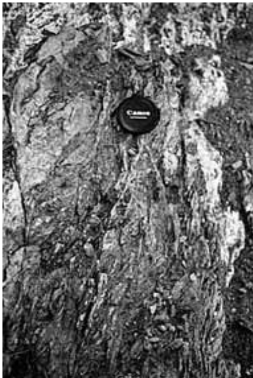
Figure 2.2 - Detailed view of the Lorca-Alhama de Murcia (LAF) fault gouge, South Bank of La Torrecilla Rambla
