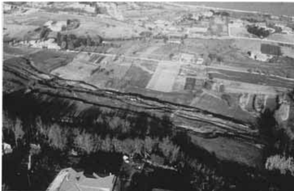
Figure 5.8 - View of the upper trench, with the main scarp in the foreground, and “antithetic” scarplets and fractures in the background.
