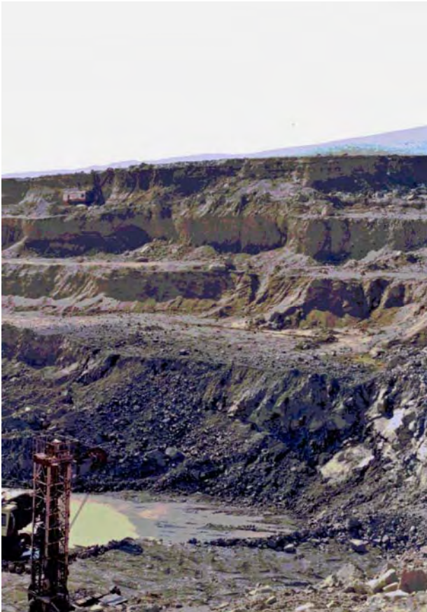
Fig. 15. The Sopcheozero chromite deposit mine, upper banks opened moraine (light colour), lower banks opened chromitite (black).
