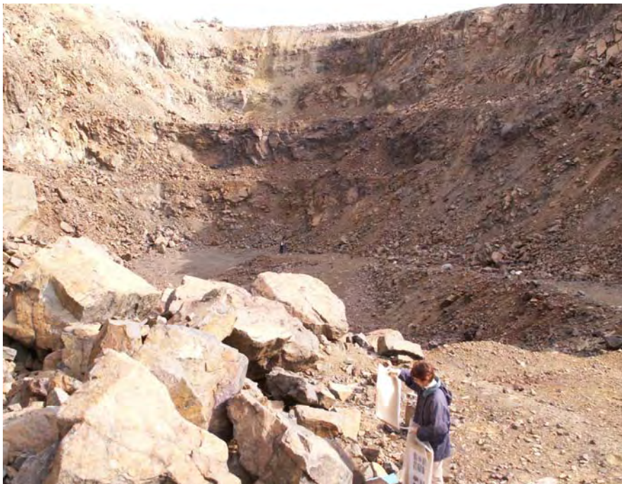
Fig.21. Mine of the Nyud-2 deposit. The walls of the mine and dumps contain numerous debris of sulphide nests and disseminated ores.
