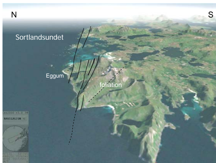
Fig. 38: 3D satellite and terrain image of the peninsula of Eggum, showing the trace of faults parallel to the West Lofoten Border Fault (lines). A zone of paragneiss is marked as foliation.
