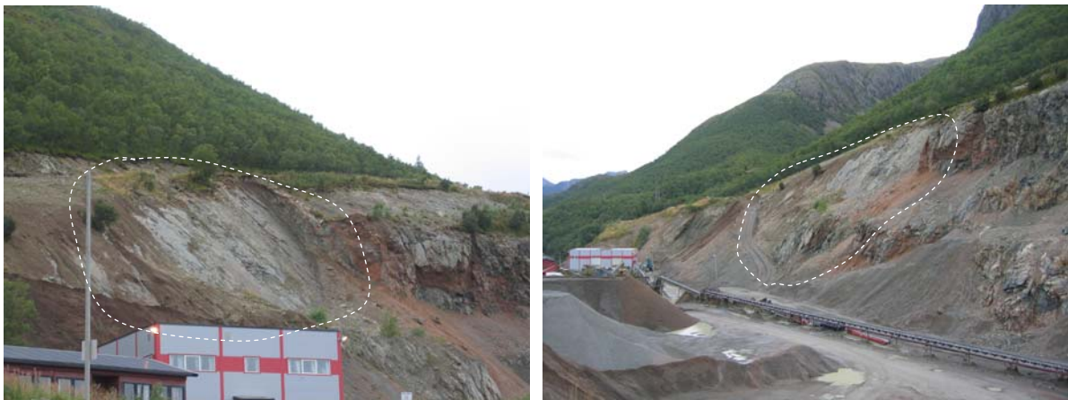
Fig. 59 : Outline of the distinct fault surface (stippled) exposed in the quarry at Rødsand. The fault is dipping c. 50 ° to the NW.
