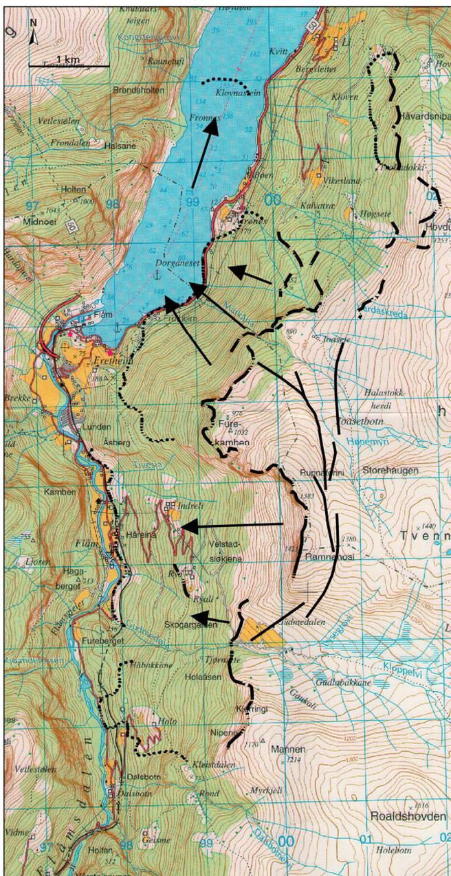
*Fig. 15. The inner part of the Aurlandsfjord and the lower Flåm valley. Old rock slide tongues and open joints representing large potential rock slides (Braathen et al. 2004).*
