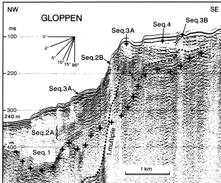
Fig. 26. Seismic profile (Sparker) of the terminal moraines and distal sediments deposited during the Younger Dryas in the Gloppen fjord. Two glacial readvances can be distinguished (Aarseth et al. 1997). +++ indicate acoustic basement (bedrock).
