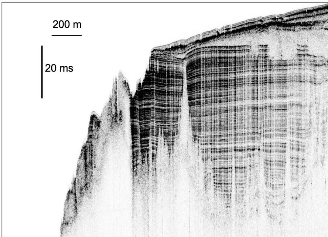
*Fig. 44. TOPAS high-resolution seismic profile from inner part of Nordfjord, showing well-laminated glacial marine sediments and acoustic transparent slide debrites above bedrock. The 1967 Nordfjord Slide have created the 15 metres high slide scar observed within the glacial marine deposits.*
