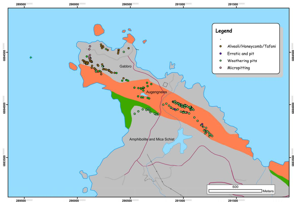
*Fig. 33. Bedrock geological map and mapped weathering pits showing the morphological dependence on lithology.*
