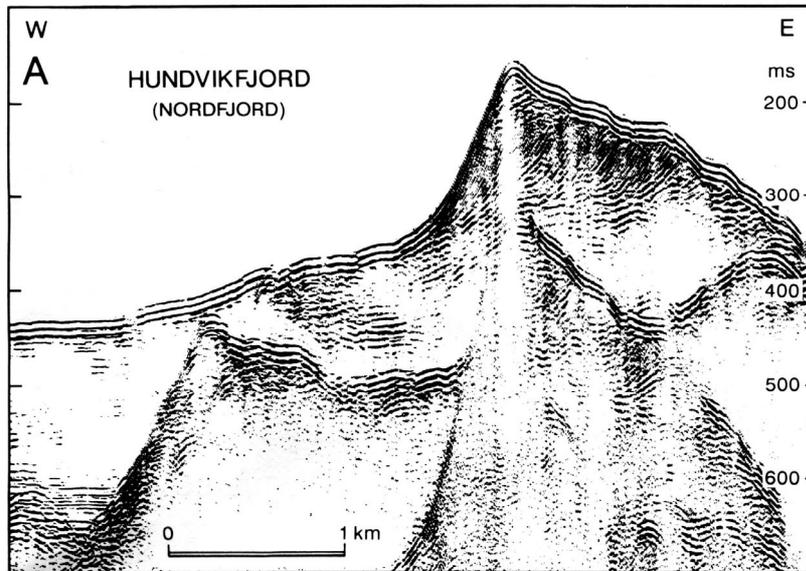
Fig. 27. Seismic profile (Sparker) across the Younger Dryas terminal moraine in the main Nordfjord. (Aarseth et al. 1997).
