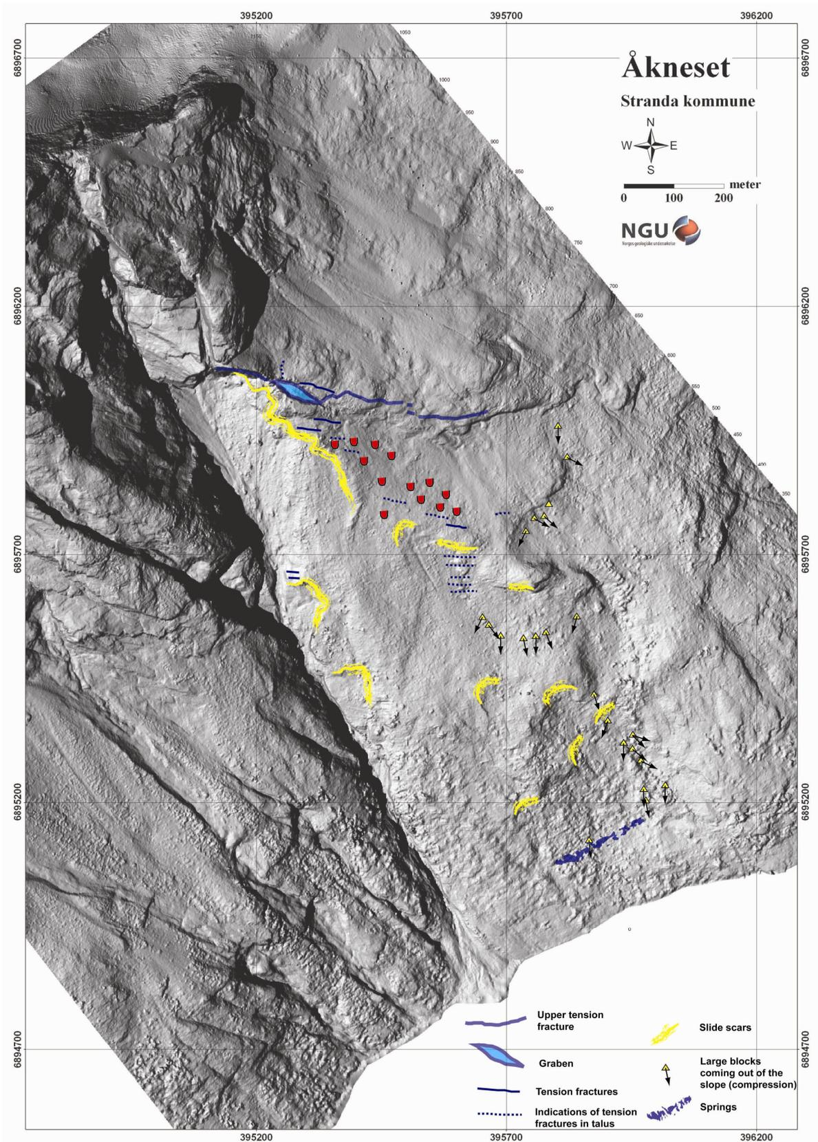
*Fig. 37. Shaded-relief map of the Åknes rockslide, with the morphological characteristics indicated.*
