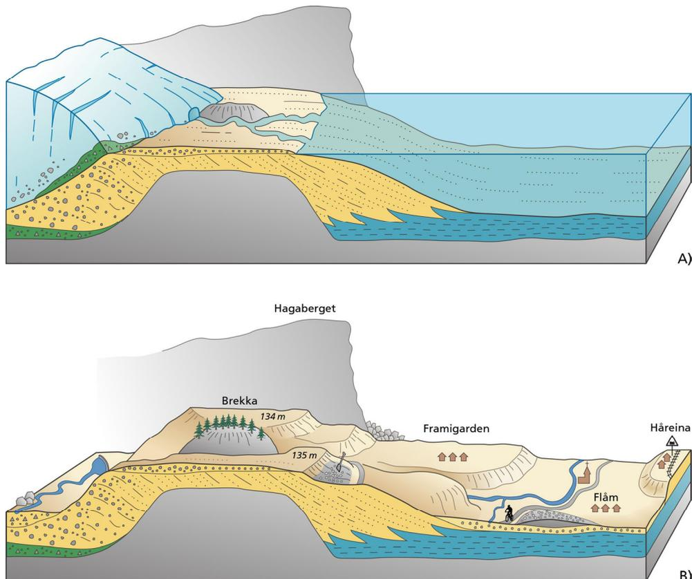
Fig. 16. Upper: Model of the deposition of a typical Preboreal icemarginal delta at the inner fjords of western Norway; example from the Flåm valley. Lower: Present day terraces with the upper marine limit at Flåm (135 m a.s.l), Aarseth et al. (2006).
