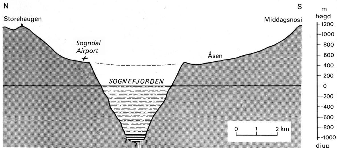
Fig. 19. Profile across the Sognefjord 15 km W of the ferry crossing Fodnes – Mannhiller. Sogndal airport is situated on the preglacial valley shoulder (Aarseth 1980.)
