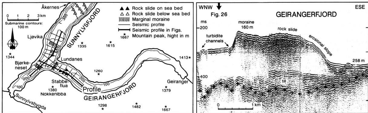
Fig. 39. Map of the inner part of the Synnølvfjord-Geirangerfjord area (left). Seismic profile (Sparker) of the Younger Dryas terminal moraine in the Geirangerfjord (right). (Aarseth et al. 1997).
