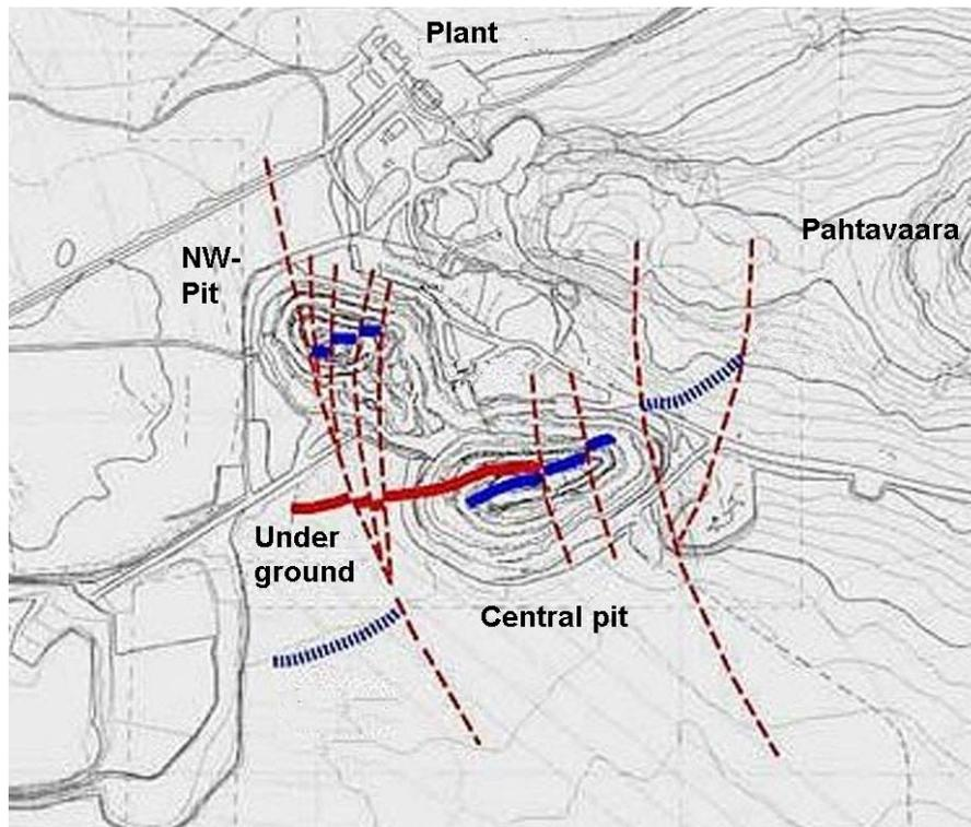
Figure 1. Map showing the Pahtavaara mine infrastructure and open cuts. Pahtavaara is a prominent hill and the landmark of the area. The rocks in the map area are Sattasvaara komatiitic rocks. Blue lines show ore mined in the open pits. The thick solid red line shows the underground resource and dashed lines cross cutting faults (Source [www.scanmining.se](http://www.scanmining.se) press release 28/04/2003).
