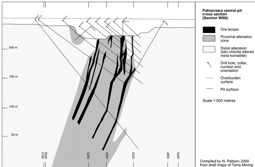
Figure 3. Cross section through the central pit of the Pahtavaara gold mine.
