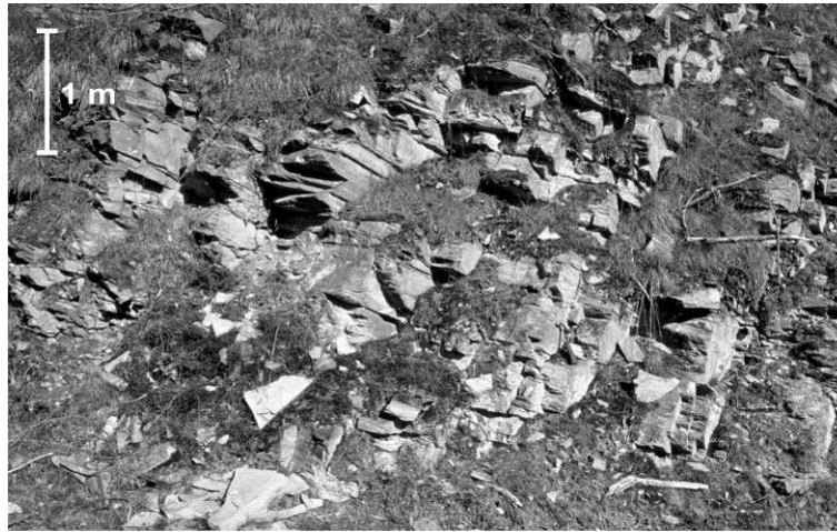
Figure 3e. Paragneiss with a closely spaced vertical NW-SE striking joint set and foliation dipping gently into the slope.
