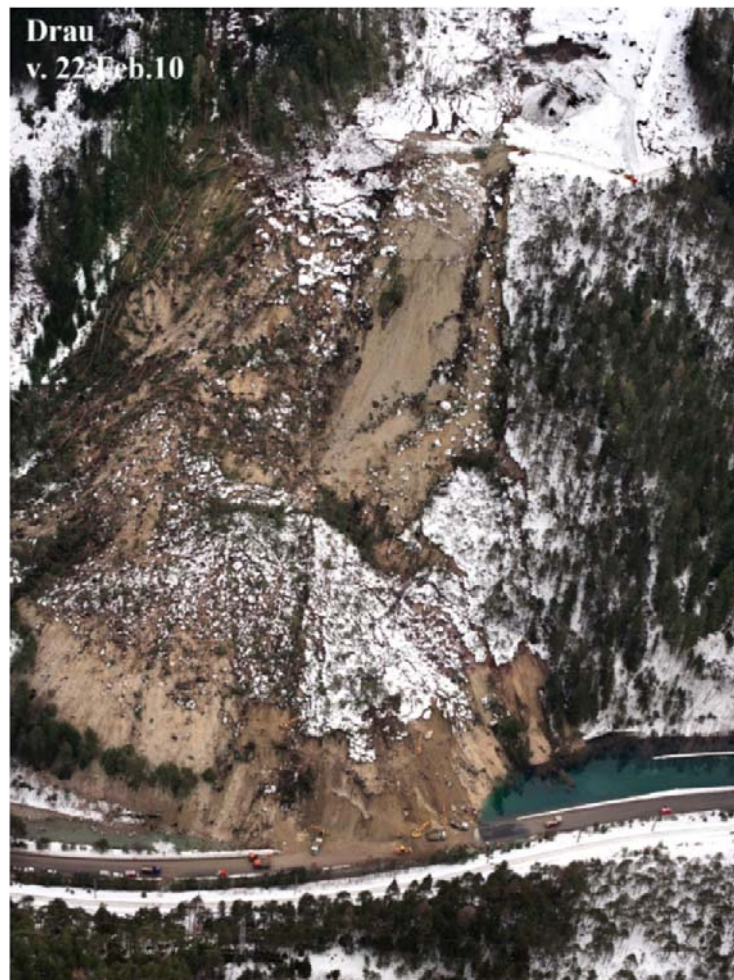
Figure 10. In February 2010 a re-activation of parts of the rockslide mass resulted again in the blockade of river Drau (picture courtesy of Baubezirksamt Lienz).
