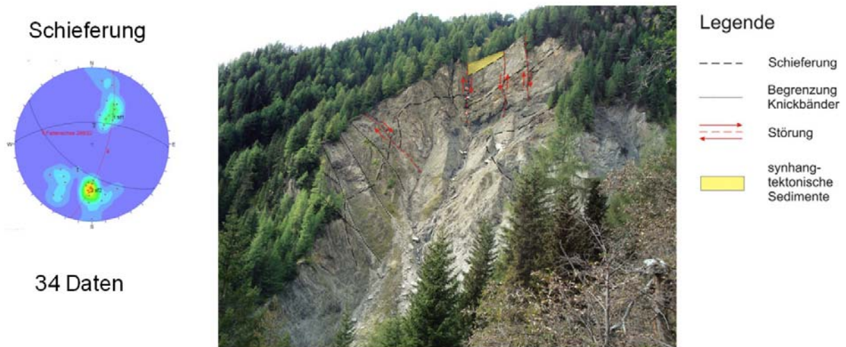
Figure 4. Region # 2, Hinge zone and Contour plot of schistosity planes; reconstruction of fold axis (stereographic projection of poles and main great circles)
