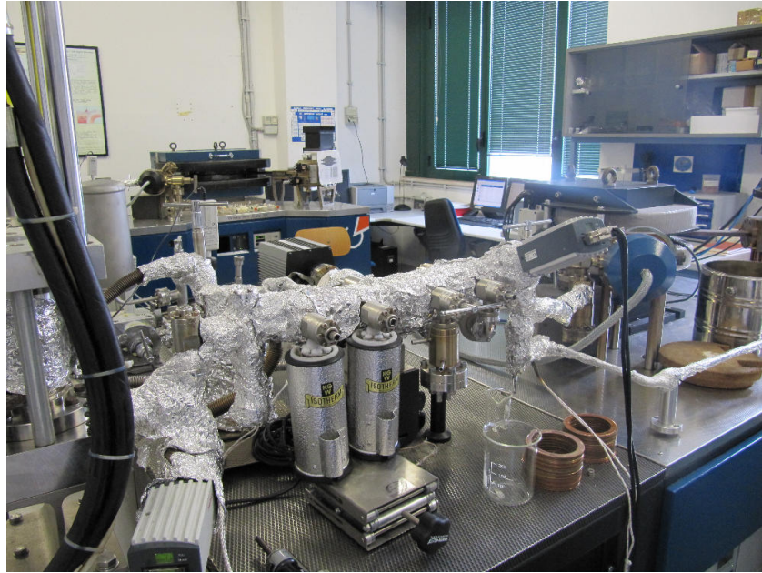
Figure 3-12: Pre-cleaning step of argon isotopes from other gases.
