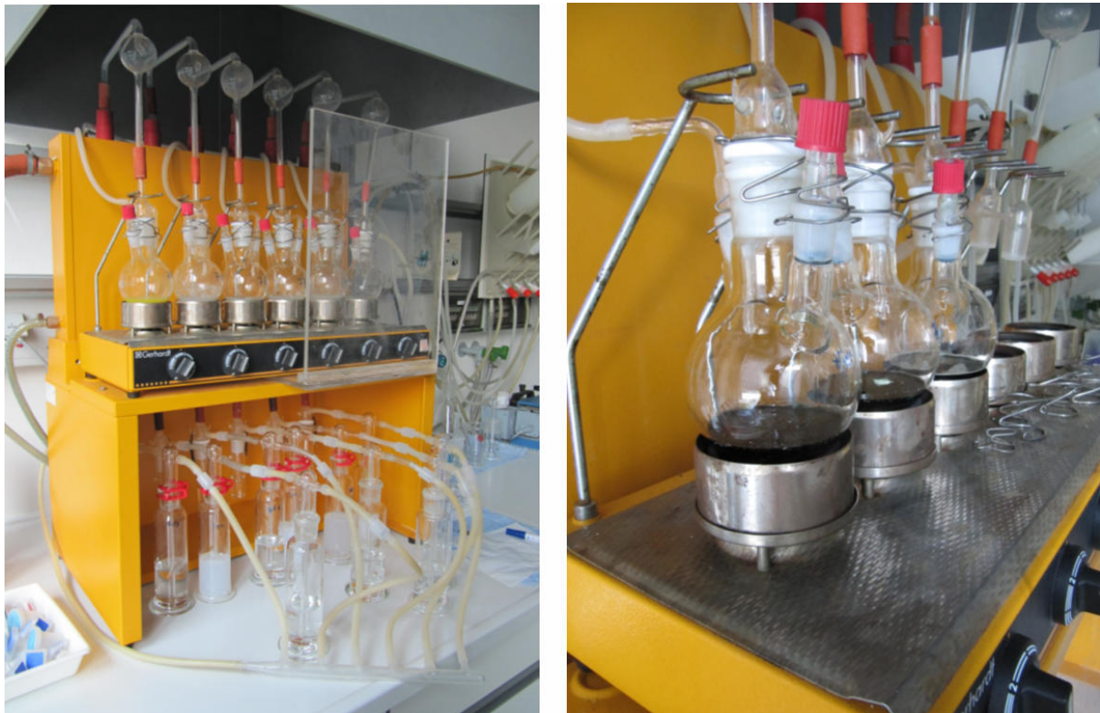
Figure 3-13: Kjeldahl distillation procedure: On the left AVS, on the right CRS with Chrom III.
