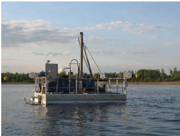
Figure 20: Base of the pilot experiment in lake Burghammer: Floating platform, CO 2 injection technology.
