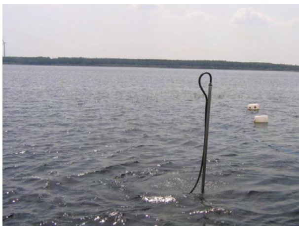
Figure 22. CO 2 gas injection lance. White buoys in background mark monitoring installations.
